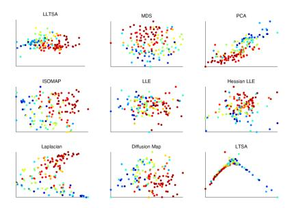
Each dot represents a city; its color – original Liveability Total score. Two axes of each sub-plot are reduced dimensions, as proposed by each method. For more details, please see the link to an MANI tool. LLTSA (linear local tangent space alignment algorithm) gives the best result here.
